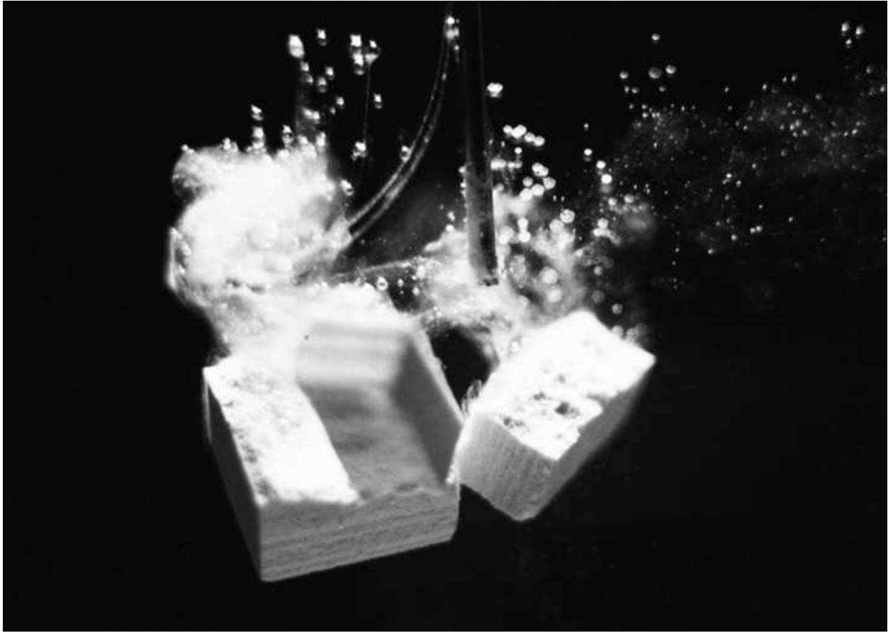
Fig. 10: Effect of a focused shock wave on an artificial stone
